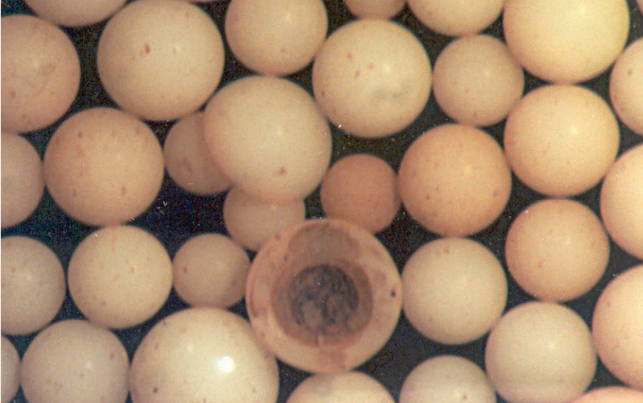
1. Iron oxide fouling of resin center
