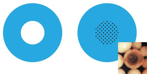
Fig. 1: A graphic depiction of an un-regenerated core with photo insert of a standard resin with a fouled center.
