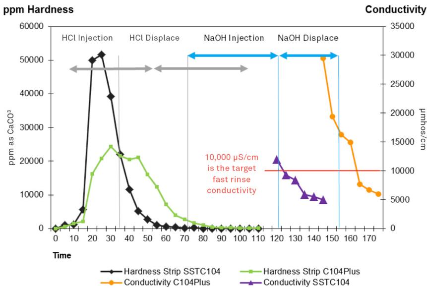
Fig. 2: A comparison between co-current regenerated WAC resin units using Shallow Shell™ SSTC104 and Purolite® C104 Plus.
