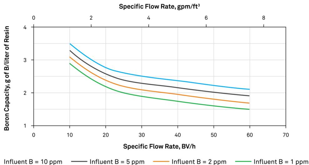
To achieve very low boron leakage, counter-flow regeneration is recommended and in some cases lead-lag operation should be considered to maximize resin capacity and achieve very low boron targets. The optimum conditions for operation and regeneration depends on the individual application.
