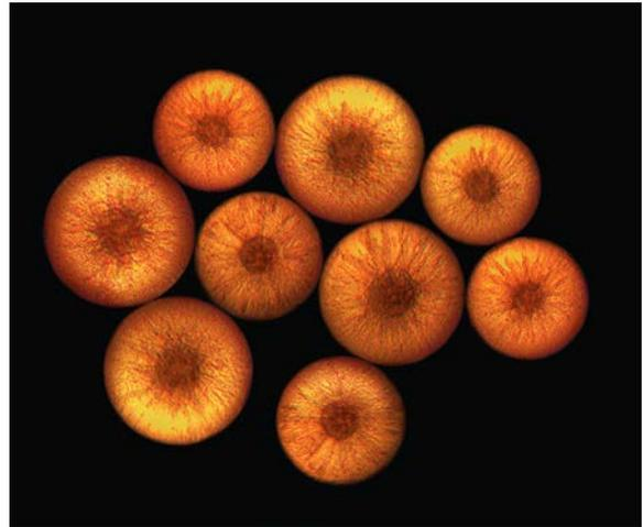
Under a microscope, Purolite SST resin looks different because each bead has an inert core that resists fouling and enables more thorough regeneration of the bead.
