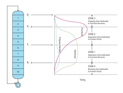
Adjustment of Inlet and Outlet Location in an SMB
