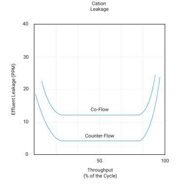
If the backwash step can be utilized infrequently, then the resin bed will be undisturbed during regeneration and a counter-flow regeneration may produce a high-quality syrup with the same throughput capacity at a somewhat lower chemical dosage. Since a weak base anion regeneration is an acid neutralization step and only a small excess of regenerant is required, no advantage is gained from counter-flow regeneration of the weak base resin.
