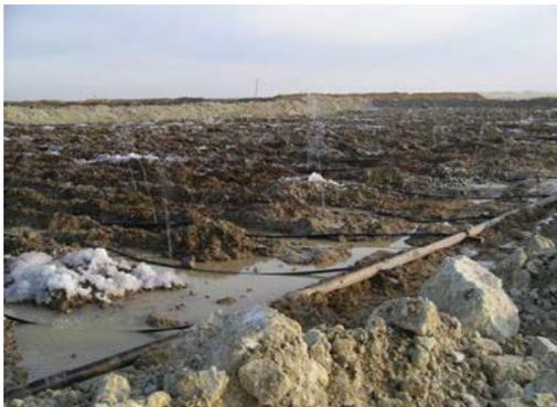
The heaps are sprinkled with lixiviant through a top distribution system.
