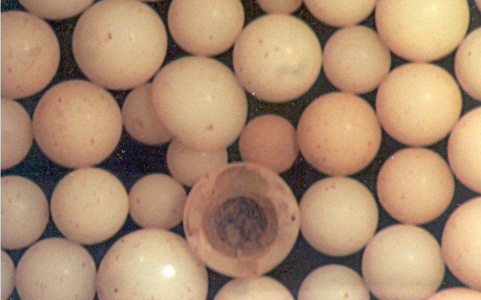
1. Iron oxide fouling of resin center
