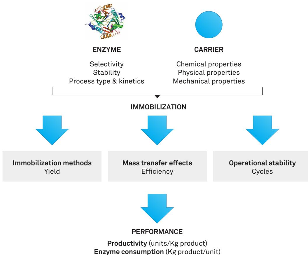
**Porosity and Surface area:** In most cases, large surface area (> 100 m<sup>2</sup>/g) and high porosity are desirable so that enzyme and substrate can be easily penetrated. Pore size of > 300 Å is usually adequate to make the internal surface accessible for immobilization of most enzymes. Lifetech ECR resins are available with different degrees of porosity and surface area, usually higher than 400Å and > 40 m<sup>2</sup>/g respectively.
