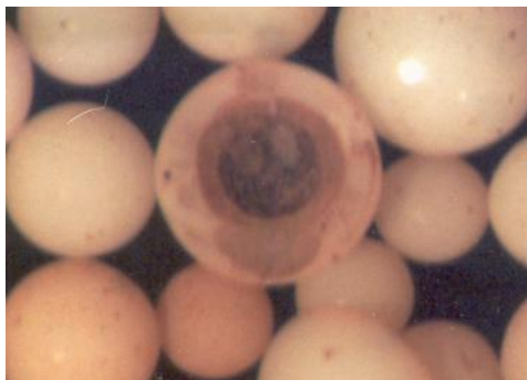
Figure 1: Standard resin with un-regenerated, (fouled) bead core
