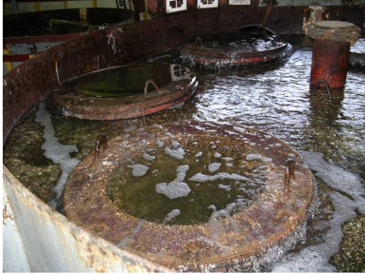
Photo 4. (left) The gold bearing cyanide solution on the top of an ion exchange column
